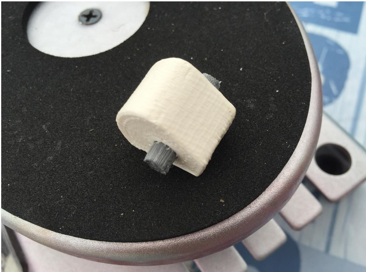
Try to get equal lengths of the axle on each side of the pivot.
