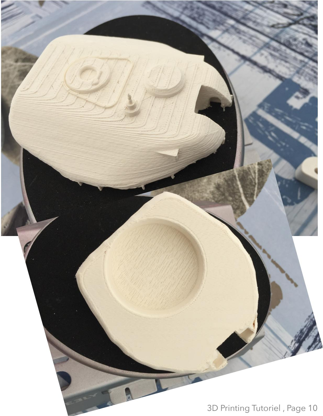
Assembly is very simple just hold the swivel upside down and the slide vertically the assemble gun and pivot into the slot, now rotate the gun to a horizontal position, this will lock the two parts together.
